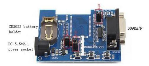
The dimension(length\*width) of board is 80\*50mm. User can power the board by DC 5V adaptor or 3V button cell(model: CR2032). When user adopts 3V button cell to power the board, user can remove short-circuiting cap from No.3 red line area to avoid power consumption by LED.
